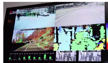
PD, TSR, Lane Detection, Sparse Optical Flow, Stereo Disparity
